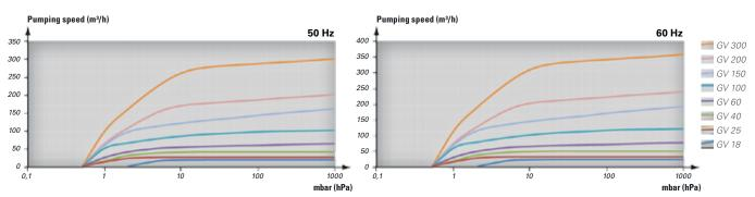
Pump performance measured at the inlet pressure and 20°C. Accuracy is +/- 10%.
